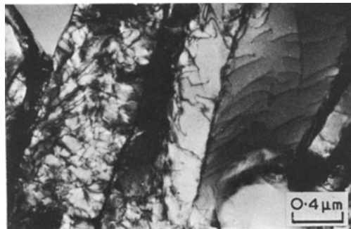
Figure 1 Single phase dislocated lath martensite structure of the beta quenched alloys.
